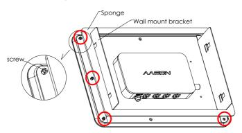
**<u>Step 4</u>**: Insert the display to the surface (opening) where you are going to mount the display
